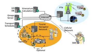
Fig.6. Architecture of the navigator service for a public transport network (PTN).
