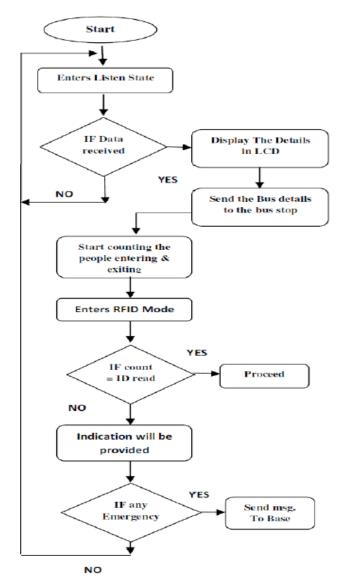
Fig. 4. Flow Chart of In Bus Module.
