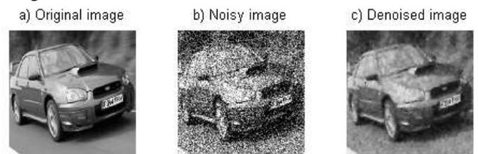
**Fig.5 Image denoised by the local adaptive wavelet image denoising technique**
