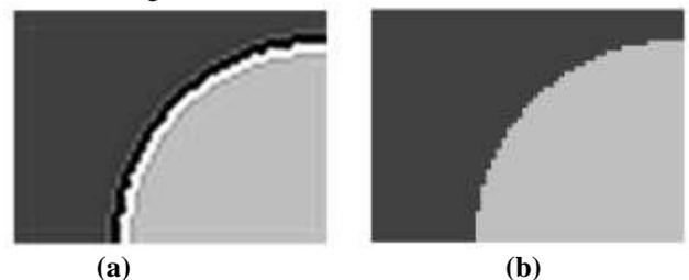
Fig. 2 a) Image with ringing effect and b) Image without ringing effect
