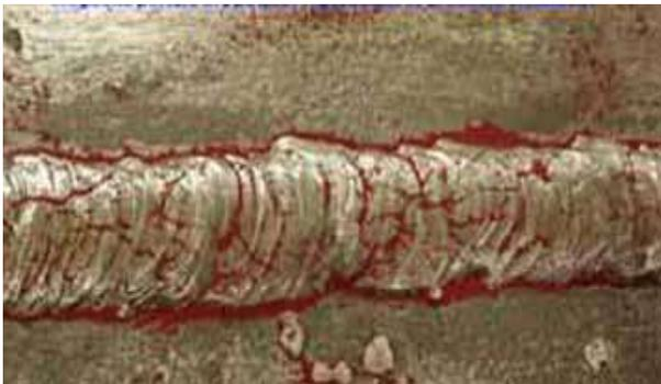
Fig-5 Indication of crack in weldments
