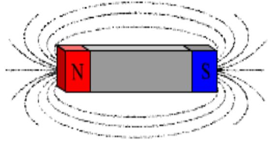
**Fig-2 Principles of MPI**
