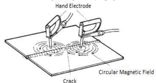
**Fig-3 Magnetization using hand held electrodes**
