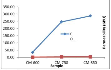
Figure 2: Comparison between CO<sub>2</sub> permeance readings with CH<sub>4</sub> permeance readings
