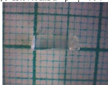
Figure :1 Photograph of single crystals of LAM
