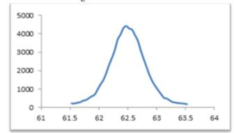
Figure 3- Gaussian function diagram on the (0112) peak for pure Titanium.
