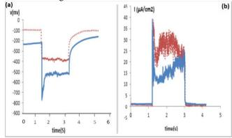
Figure 3-diagram of tribocorrosion test under a) open circuit b) anodic conditions for uncoated and coated 316L stainless steel in Ringer's solution.
