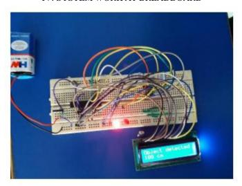
IN this project if any object come across the project at a distance 180cm then it detects and buzzer are work at alarm function. For **E.g.** in the figure any object come at project distance then its detect and show the how long distance.
