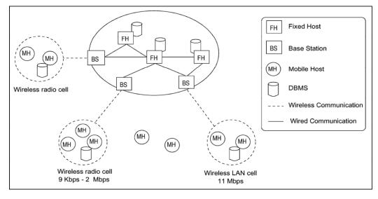
Figure 1. Architecture of mobile database systems
