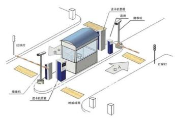
Radio Frequency Identification (RFID) technology is very useful technology in automation of vehicle parking in office complexes and other locations such as malls and other buildings.
