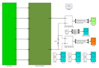
Fig. 5. Seven Level Single Phase Inverter Model in MATLAB Simulink
