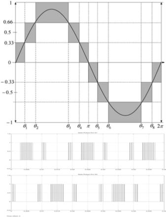
Fig. 9. PWM signals for S1 and S3.
