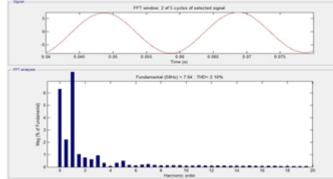
Fig. 16. THD Analysis of current waveform in case of RL Load.
