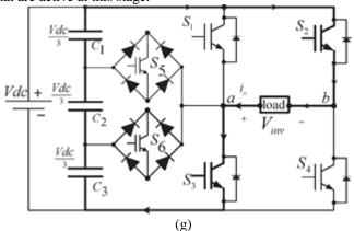
Fig. 2. (Continued.) Switching combination required to generate the output voltage (Vab). (c) Vab = Vdc/3. (d) Vab = 0. (e) Vab = -Vdc/3. (f) Vab = -2Vdc/3. (g) Vab = -Vdc.
