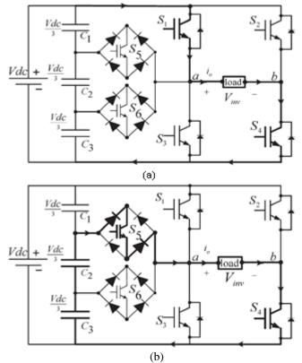
Fig. 2. Switching combination required to generate the output voltage (Vab). (a) Vab = Vdc. (b) Vab = 2Vdc/3.
