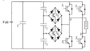
Fig. 1. Proposed single-phase seven-level inverter with modified H-bridge topology
