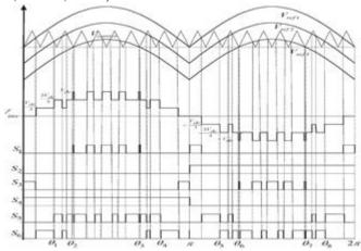
Fig. 3. Switching pattern for the single-phase seven-level inverter
