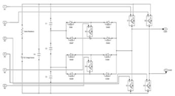
Fig. 6. Seven Level Diode-Clamped Cascaded Inverter
