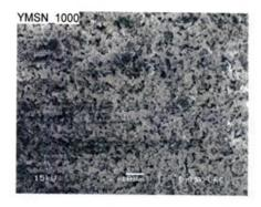
Fig.5(c). SEM image of palm shell bio-char at 1000 °C for 2 h
