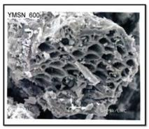
Fig.5(a). SEM image of palm shell bio-char at 600 °C
