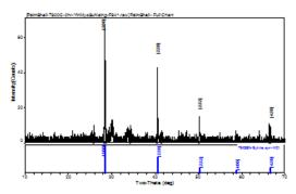
Fig.3(b). The XRD pattern of palm shell bio-char at 800 °C for 2h
