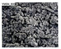
Fig.5(b). SEM image of palm shell bio-char at 800 °C for 2 h
