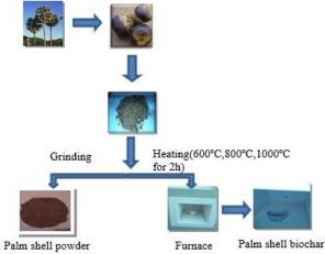
Fig.1. Block diagram for experimental procedure of palm shell biochar.
