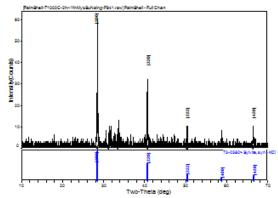
Fig.3(c). The XRD pattern of palm shell bio-char at 1000 °C for 2h
