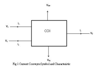
The current conveyor's response is given by equat ion
