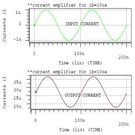
Fig. 7 Transient analysis for current amplifier
