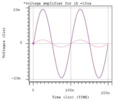
Fig. 4 Graph for Transient Response of Amplifier for f=10MHz
