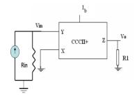
Fig.6 Circuit of Tunable Current Amplifier
