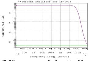
Fig 8 Frequency response for Current Amplifier
