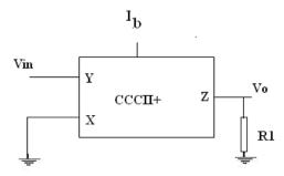
Fig.3 Circuit of Tunable Voltage Amplifier
