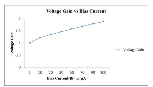
Fig. 9. Graph between Voltage Gain & Bias Current, R1=1K constant
