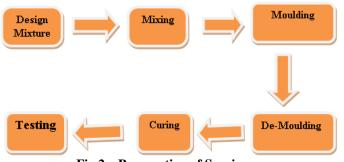
Fig.2 Preparation of Specimen
