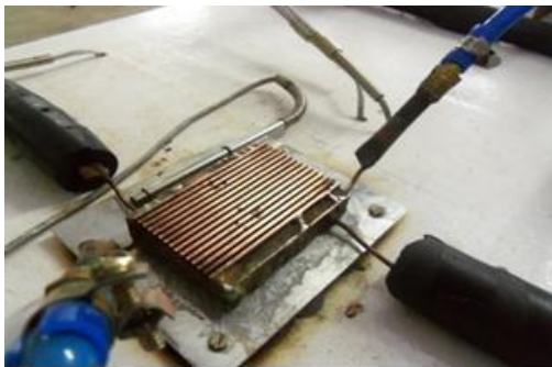
Fig.2. Core section of the microchannel with fin
