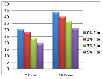
Fig 5.2 Compressive strength comparison of cubes of different percentage
