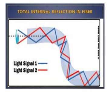
Fig 2.1 Total internal reflection in fibers
