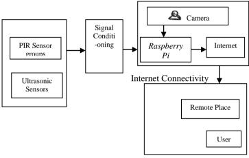
Figure 1. Use of smart sensors to improve the sensing reliability of an embedded surveillance system
