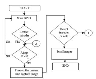
Figure 2. Detection software flowchart
