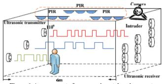
Figure 6. Arrangement of our experimental environment.
