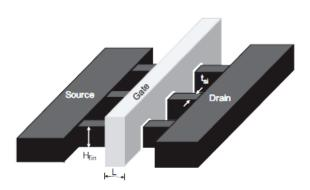
Fig 7. Three – FinFET.  $W_{total} = 3 \times (2 \times H_{fin} + t_{si})$ .
