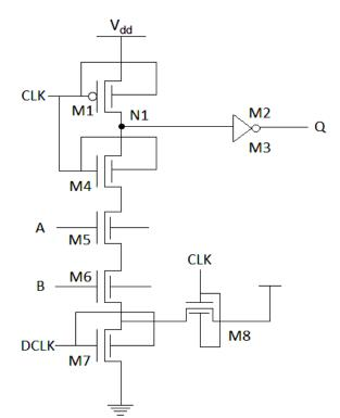
Fig 12: Proposed Technique AND Independent Gate using FinFET.
