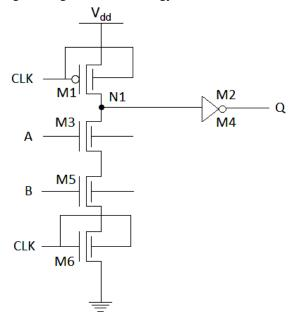
Fig. 10. Domino AND Independent Gate using FinFET.
