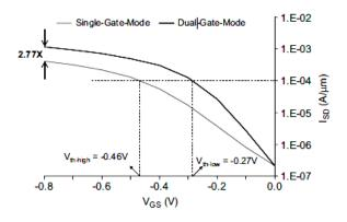
Fig. 8. Drain current characteristics of a single-fin P-type IG-FinFET. The source-to- drain voltage is 0.8V. T = 110 1C. I off = 216nA/mm. Ion (single-gate-mode) = 0.422 mA/um. Ion (dual-gate-mode) = 1.17mA/um. The threshold voltage is the gate-to- source voltage at which the drain current per fin height is $10^{-4}$  A/um for |VDS| = VDD.
