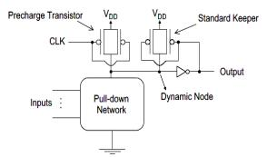
Fig. 9. A standard footless domino circuit in a tied-gate FinFET technology.
