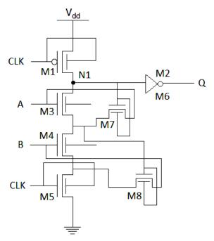
Fig 11. Twin Transistor AND Independent Gate using FinFET.
