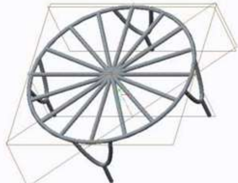
Figure 3 : Support stand designed with help of Creo and manufactured of Steel Bars
