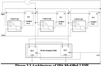
Figure 3.3 Architecture of 3Bit Modified LFSR
