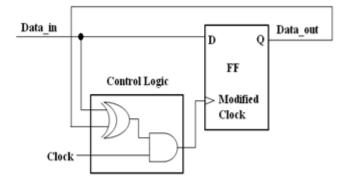
Figure 3.2 Switching unit of LFSR with Modified Clock
