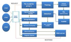
Figure 1.2: Architecture of proposed system.
