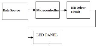
Fig. 6 VLC Transmission Part
