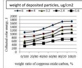
Fig. 8 the extent of collected solar heat as a function of the weight ratio of carbon/cuprous oxide/composite on the glass surface.
