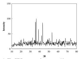
Fig. 6a The XRD pattern of cuprous oxide prepared by reduction of copper nitrate with hydrazine hydrate
