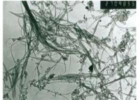
Fig. 1 Carbon single walled nano tubes (after ref.15)
