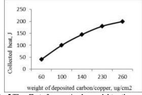
Fig. 5 The effect of copper/carbon weight ration on the extent of the collected solar heat
