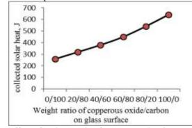
Fig. 7 Effect of weight ratio of cuprous oxide / carbon of the deposited carbon particles (on glass surface) on the extent of the collected solar heat.
