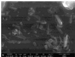
Fig. 3 FE-SEM photograph of the prepared carbon nanotubes.
