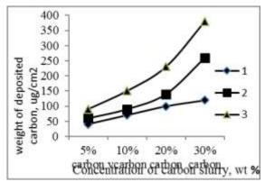
Fig. 4 weight of carbon nanoparticles deposit on glass surface as affected by number of application and concentration of carbon in slurry.
