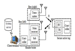
Figure: Block Diagram of Active RFID Active RFID tags are basically miniature radio flares and contain both a radio transmitter and a radio receiver circuit. An Active RFID tag consists of three main parts: tags, readers and servers.
