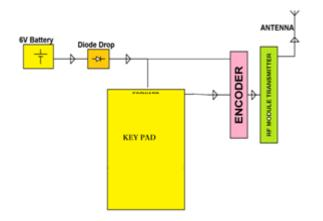
The active RFID tags have their own source of power. They can transmit stronger signals over long distances and can operate in rugged environment for many years. Because of the on- board source of power they are larger in size and
