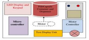
Figure 1 Block Diagram of Medication Dispenser
