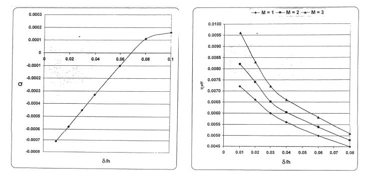
Graph - 1.2:Variation of flow rate with PPL thicknessGraph - 1.4:Variation of effective viscosity with PPL<br/>thickness. $(m \rightarrow 0)$ .thickness.
