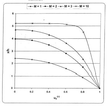
**Graph – 1.7:** Variation of velocity for different values of PPL thickness..
