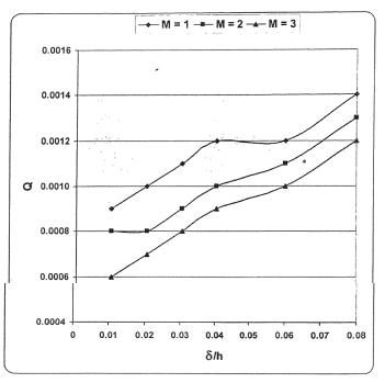
**Graph – 1.1:** Variation of flow rate with PPL thickness.
