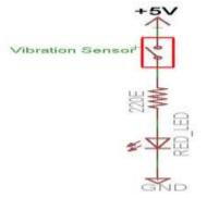
Fig7: Diagram of vibration sensor
