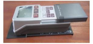
Figure 2: Talysurf (Surface roughness tester Model: SJ-301)
