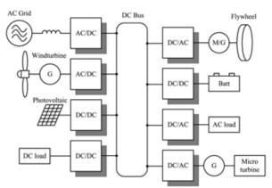
Fig. 1. Conceptual diagram of a dc-bus microgrid system.
