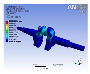
Fig. 5 Equivalent elastic strain of Structural steel crankshaft
