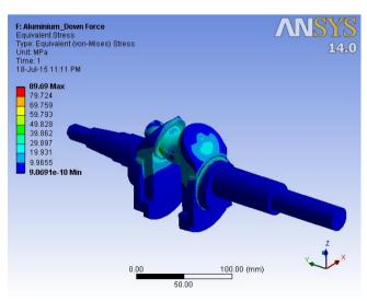
Fig. .4Von Mise's Stress of Al 5083 alloy Composite Crankshaft
