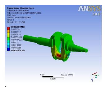
Fig.8 Total Deformation of Al 5083 Composite Crankshaft
