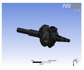
Fig.2Meshed Model of Crankshaft
