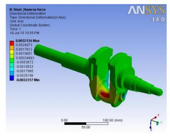
Fig.7 Total Deformation of Structure steel Crankshaft
