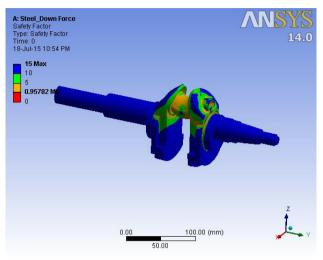
Fig.11 Safety Factor for Steel
