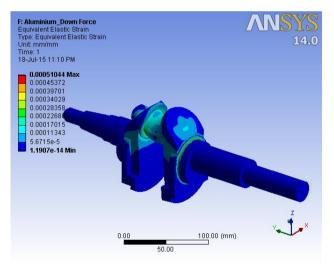
Fig. 6 Equivalent elastic strain of Al 5083 alloy Composite Crankshaft
